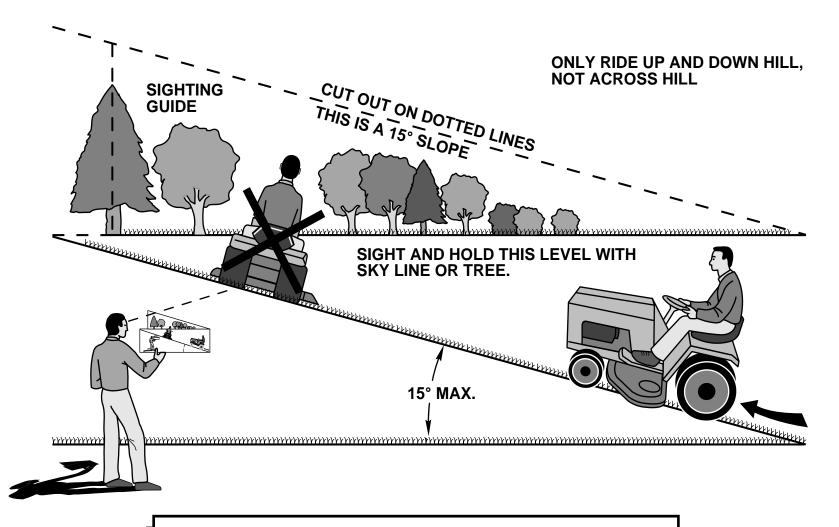
Operate your Tractor up and down the face of slopes (not greater than 15°), never across the face. Make turns gradually to prevent tipping or loss of control. Exercise extreme caution when changing direction on slopes.
